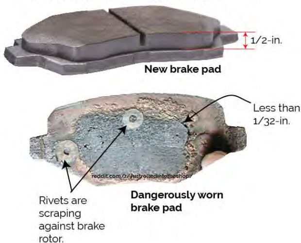
New brake pad versus worn brake pad
