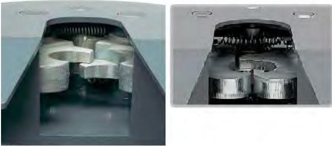
Fifth Wheel Locking Jaws: OPEN CLOSED
