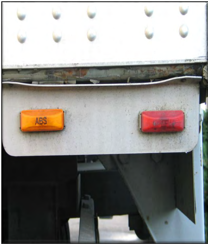
Figure 6.7 – ABS Malfunction warning Light.
