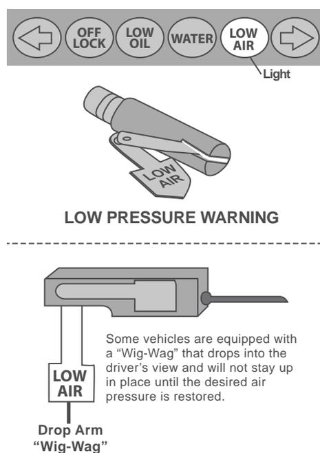
If the warning signal doesn't work, you could lose air pressure and you would not know it. This could cause sudden emergency braking in a single-circuit air system. In dual systems the stopping distance will be increased. Only limited braking can be done before the spring brakes come on.
