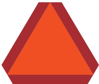
*This safety device is required on all slow-moving (25 mph or less) vehicles. Here's how this SMV emblem can protect you ...*
