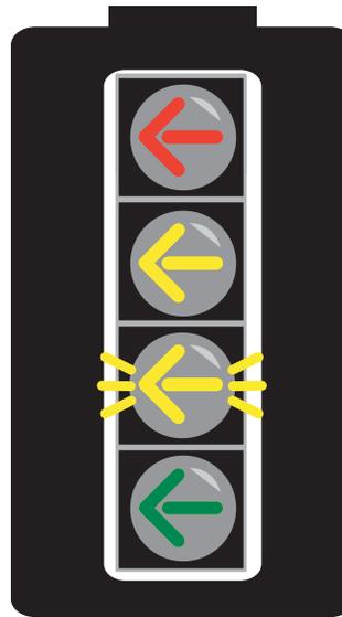
The new left-turn signal head has four signals.
