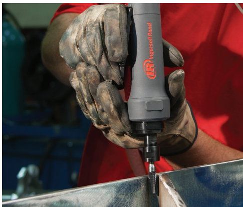
Weld cleaning and smoothing
