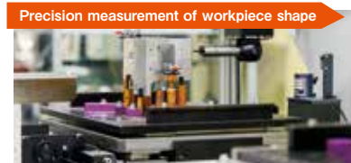
Coordinate measurement is performed with MiSTAR 555. Shape details that cannot be measured with a gage will be quantified.
