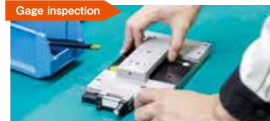
Workers measure workpieces with a dedicated gage to check whether their dimensions are correct as specified in the drawing.
