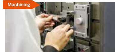
Components of the coordinate measuring machine are prepared at this stage. They are automatically processed by multiple machining tools and then deburred and cleaned by workers.
