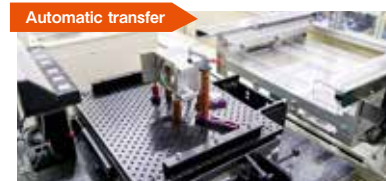
A set workpiece is automatically transferred to the measuring machine as scheduled. Workers are released after setting the workpiece and do not have to wait during measurement.
