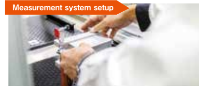
Workers set a workpiece in the jig on the measurement system at the right time. Each workpiece is identified by its QR code.
