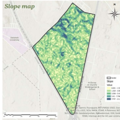
1. Slope Map – Determines safe construction locations and areas to be left as green spaces.
