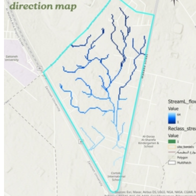
8. Stream Flow Map – Determines precise water flow paths → Helps design natural agricultural and watershed areas.
