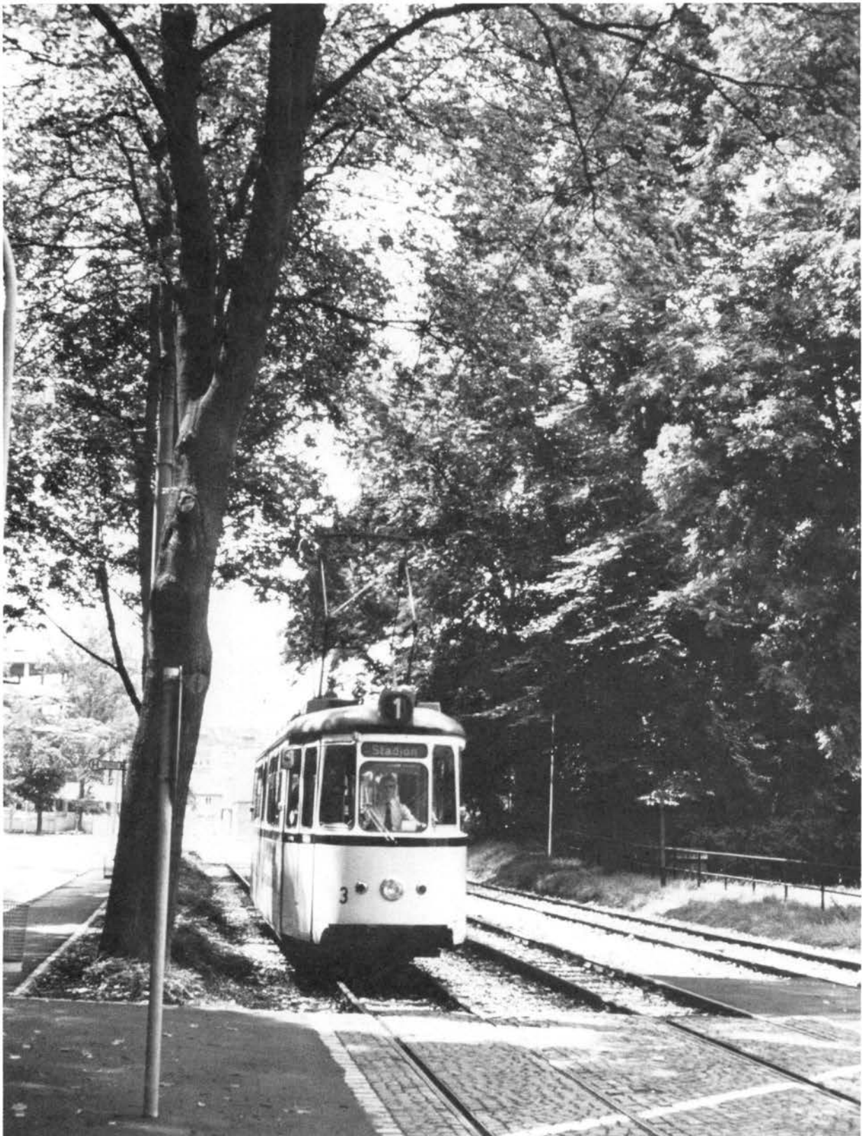
Figure 7. Landscaping used to make the overhead less noticeable.
