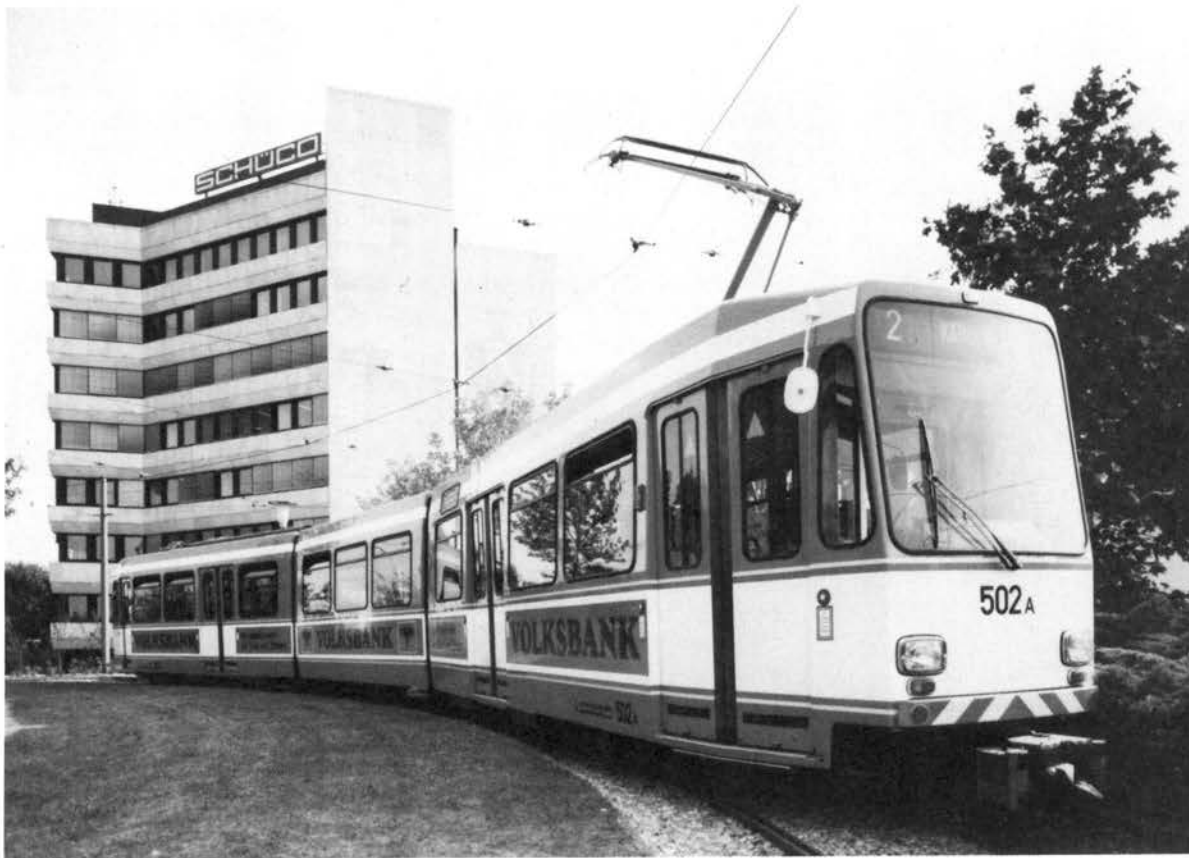
Figure 2. Light rail vehicle. The ability to bend with the curvature of the track is demonstrated by this double articulated car.
