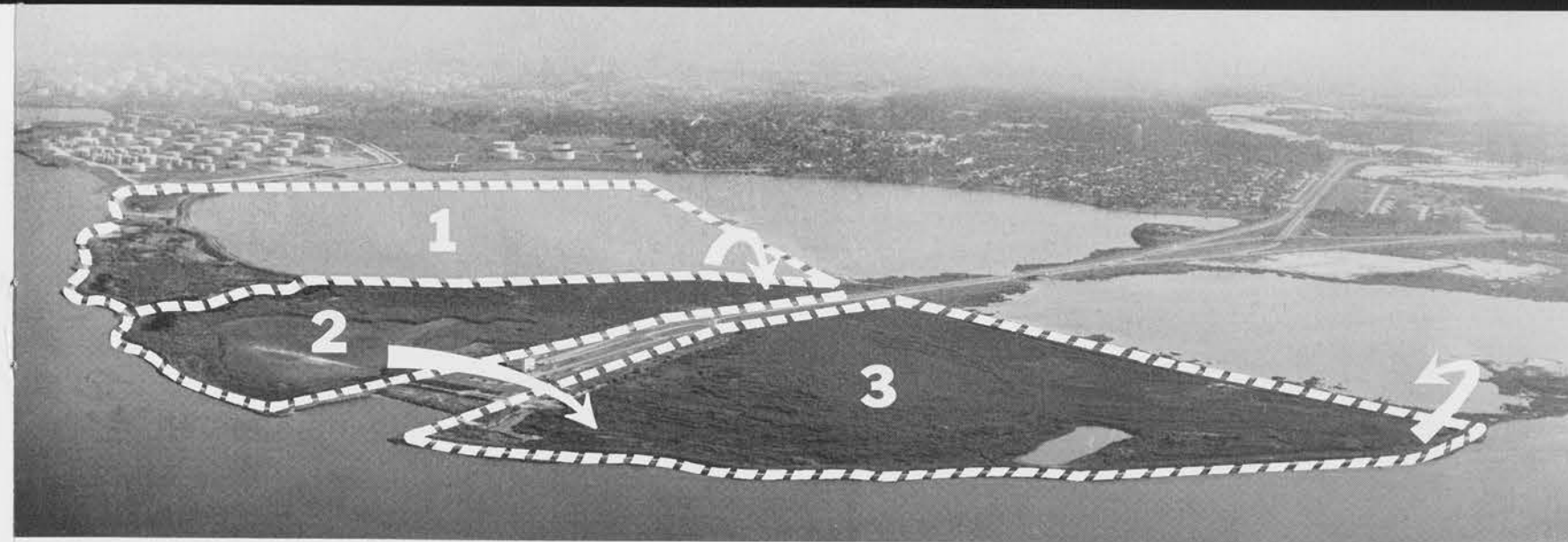
Within the dotted lines on this aerial photograph are the three sections that make up Baytown Refinery's 380-acre ponding system. After the effluent level builds up in Section 1, it will flow, as indicated by arrows, into Sections 2 and 3 (now dry as shown) before it is finally discharged into the Houston Ship Channel. Total retention time of effluent in the ponding system: 45 days.
