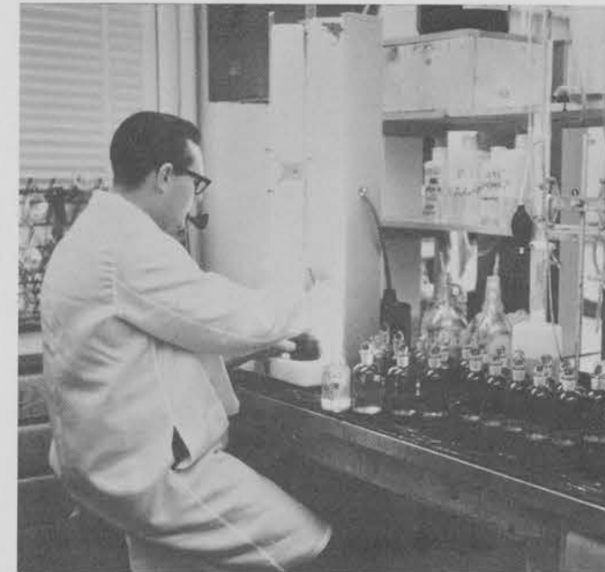
A chemist at the Minneapolis Office of the Federal Water Pollution Control Administration analyzes water samples for dissolved oxygen.
