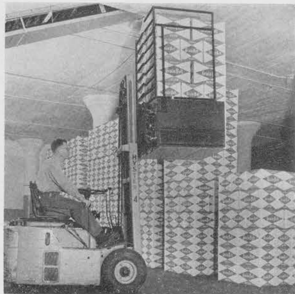
Lift truck, equipped with hydraulic grab arms, easily places load at elevated height.
