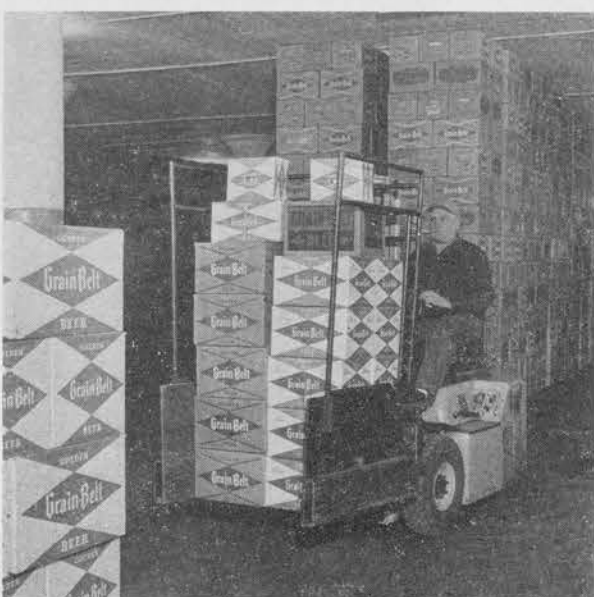
The hydraulic grab arms also handle miscellaneous loads of varying sizes.
