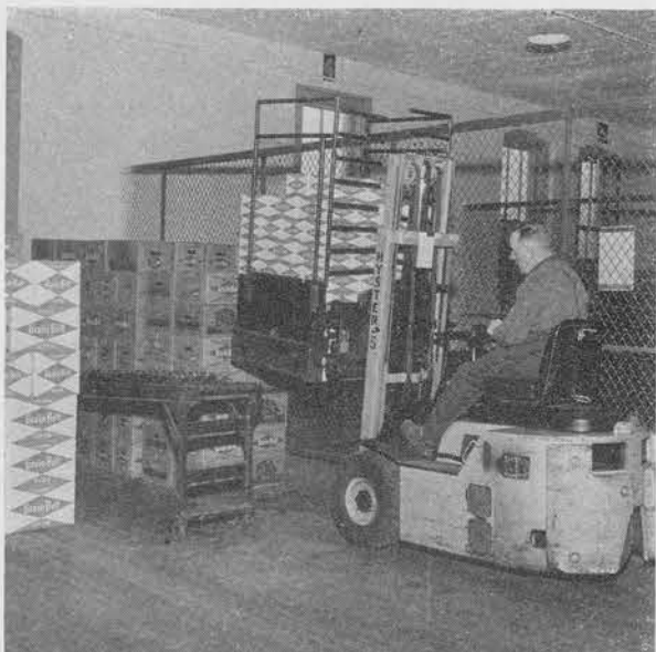
Hydraulic side shift enables alignment of loads, both vertically and horizontally, without "jockeying."
