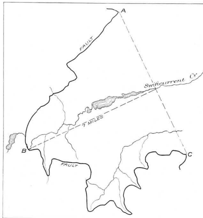
FIG. 15.—DIAGRAM ILLUSTRATING THE METHOD BY WHICH THE AMOUNT OF VISIBLE OVERTHRUST ON SWIFTCURRENT CREEK WAS DETERMINED.
