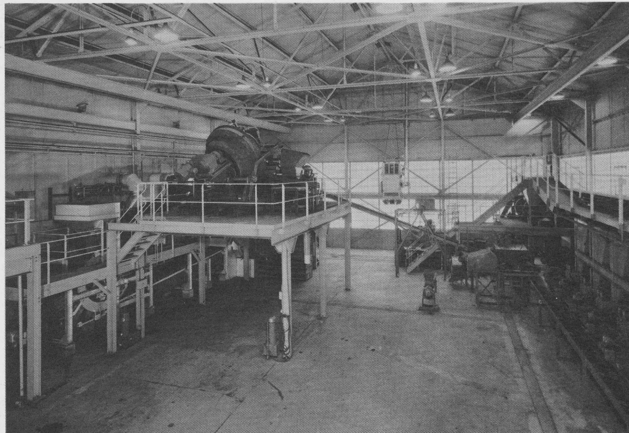
An overall view of the sintering section of the Laboratories. Materials to be tested are fed onto collecting belt from the bins shown at the right, and are fed onto the up-sloping conveyor that crosses the rear of the photo. Next they are automatically weighed by the ABCs Scale,
