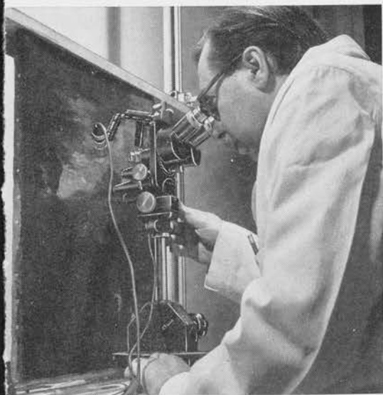
Instrumentation, art-chemist style: mobile binocular microscope on vertical frame expedites Dr. Nathan Stolow's examination of surface of old painting. Below: assistant uses instrument that measures dynamic film dimensions in study of action of new solvents on drying oil films.
