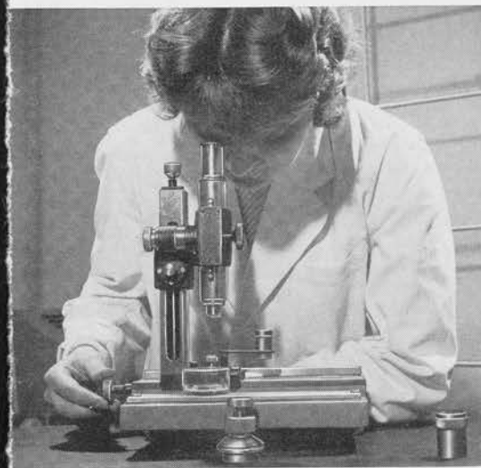
Instrumentation, art-chemist style: mobile binocular microscope on vertical frame expedites Dr. Nathan Stolow's examination of surface of old painting. Below: assistant uses instrument that measures dynamic film dimensions in study of action of new solvents on drying oil films.
