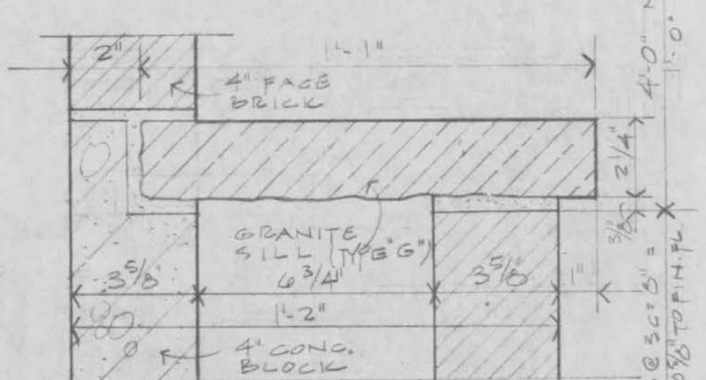
SILL DETAIL FIRE EXTINGUISHER NICHE SCALE 3/8" = 1'-0"
