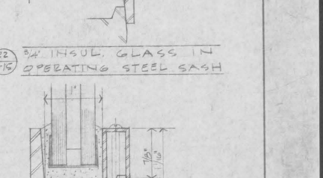
26 SECOND FLOOR CASEMENT DETS - WINDOW PANEL 5 SCALE: 3/4" = 1'-0"
