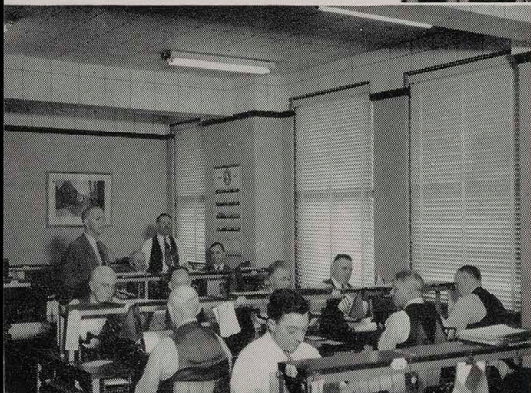
Acoustically treated ceiling absorbs noise from telegraph instruments and typewriters. Fluorescent lighting provides daylight working conditions around the clock. Ivory colored venetian blinds enhance the appearance of the modernized relay office
