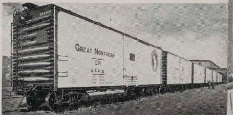
Great Northern pioneered quantity construction of plywood-steel freight cars. Light, but sturdy, these cars are ideal for grain, forest products and merchandise.
