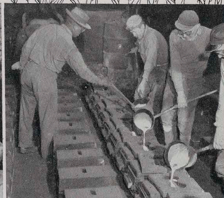
Linseed oil is used to bind fine sands for foundry molds from which castings for many types of machinery are produced
