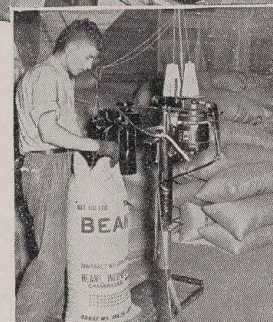
An automatically controlled chute and scale fills and weighs bags of 100 pounds each which are then sewed up by a power machine
