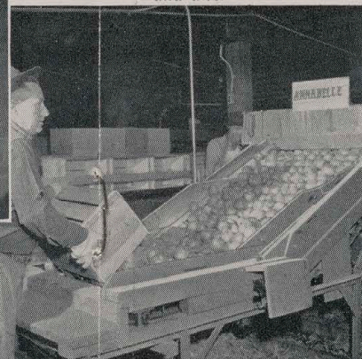
Big washing machines using hot and then cold water remove spray and dirt.
