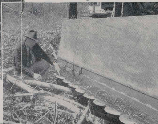
Harry J. Johnson, fieldman for the Iron Range Resources and Rehabilitation office, indicates heavy cutting edge at the bottom of the land clearing machine.
