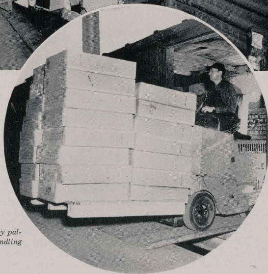
Palletizing is most effective for shipments of uniform size. Loading is quick and easy with mechanical transporters.
