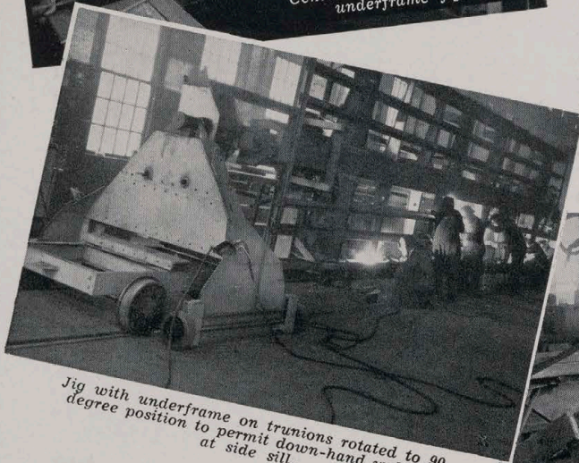
Center sill assemblies with underframe jigs.
