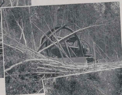
Large Steel bars protect the machine and the operator.
