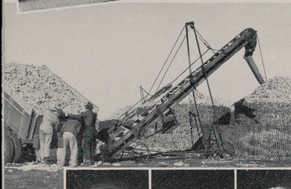
Power conveyors unload eared corn from trucks into cribs each holding 600 bushels
