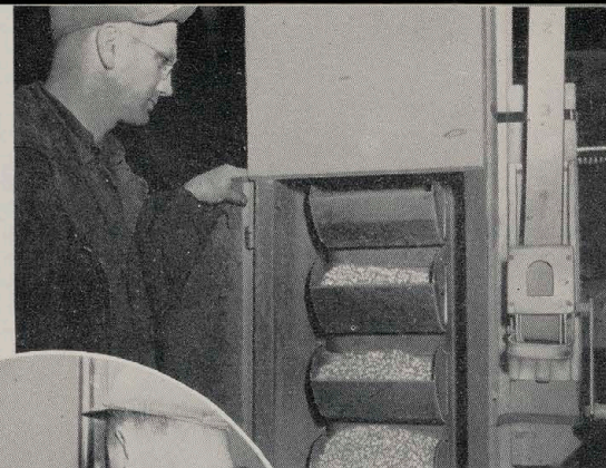
A power lift carries shelled corn from bins to top of elevator where a long chute takes it to drying plant
