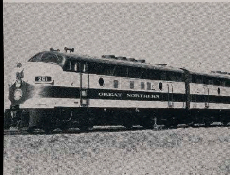
Two-unit 3,000-horsepower diesel-electric passenger locomotive.
