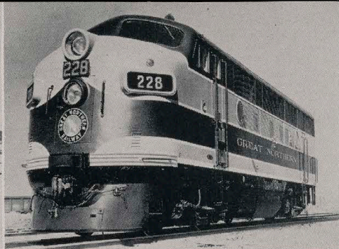
Single-unit 1,500-horsepower diesel-electric locomotive.
