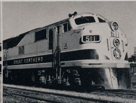
Single-unit 2,000-horsepower diesel-electric locomotive.
