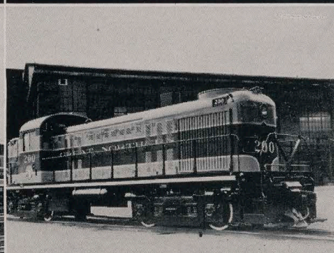
1,500-horsepower diesel locomotive for road work at various points on GN.
