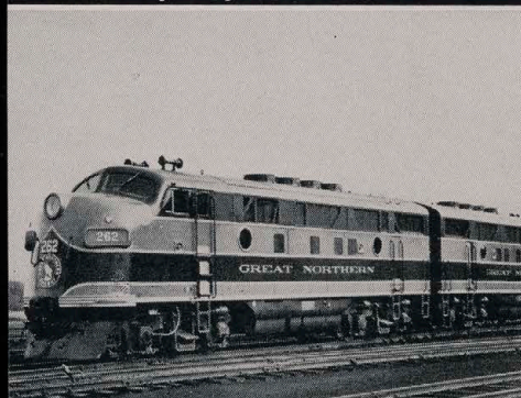
Two-unit 3,000-horsepower diesel-electric freight locomotive.
