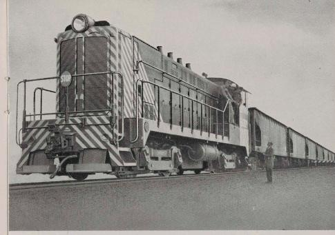
One of the 120-ton diesel electric locomotives operated by Hanford Works railroad.
