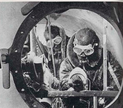
In the Stratochamber, Boeing engineers bring the stratosphere down to sea level as part of their high-altitude research.
