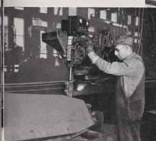
Automatic welding of body bolster section by the submerged arc process.
