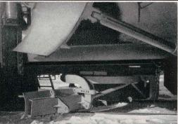
Mechanism which permits change of scraper angle, horizontally and vertically.
