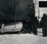
Flanger blade at rear of dozer, shown in raised position.
