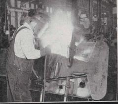
Body bolster sections, positioned in the jig, are tack-welded by hand.
