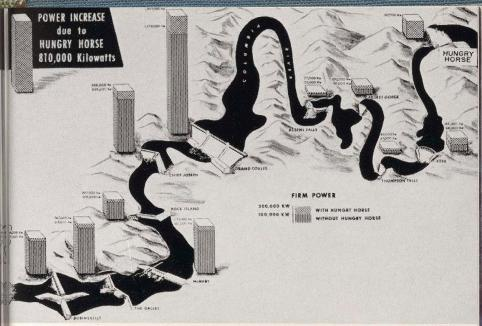
Map illustrates graphically how the year-around firm power-producing capacity of downstream dams is increased with the completion of Hungry Horse Dam.
