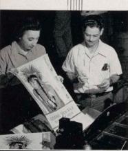
Tinning top and bottom of calendars is one of the final phases of production.
