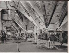
Twelve digesters are in operation during manufacture of high quality bleached sulphite pulp.
