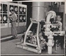
Master control panel for stock meters which deliver material to the mixing chest. Times photo.
