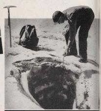
Thickness measurements are taken through natural holes called "Moulins" or "ice wells".
