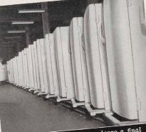
Completed refrigerators undergo a final inspection before being crated.
