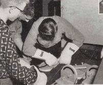
Left to right. James Stack, Floyd Clasen and James Froelke insert heated plastic frame strips into wooden jigs.
