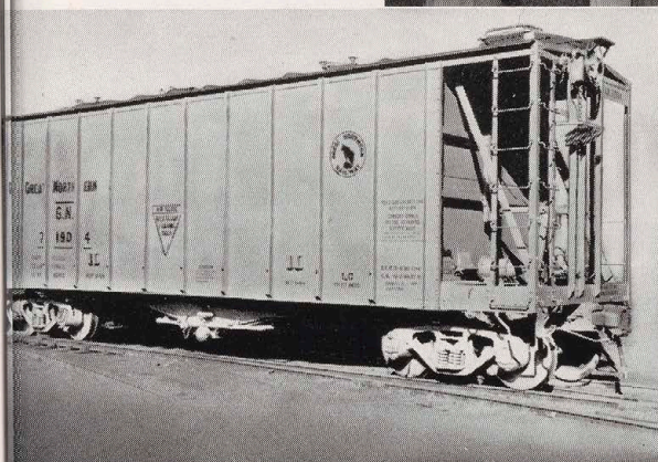
"Airs- lide" hopper car, one of several purchased by Great Northern Rail- way to facilitate ship- ment of flour, sugar and other commodities in bulk.
