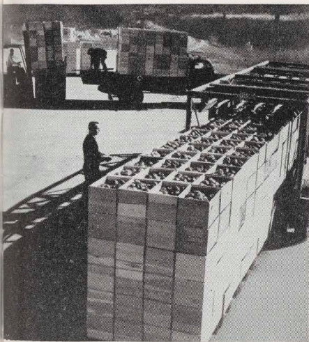
Becoming popular as a means of transportation between orchard and packing plant is the use of "hyster" equipment. Regular box pallets as well as tote bins can be accommodated.
