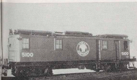
The world's most powerful single cab electric locomotives were used in the Cascade Tunnel prior to ventilation which permits diesel-electric operation.
