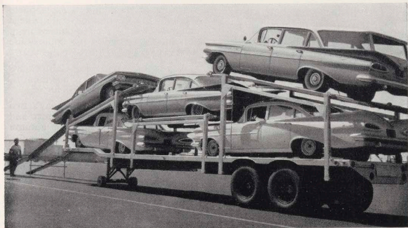
The Great Northern Railway has purchased similar piggyback equipment as shown above for the installation on flat cars. Two will be mounted on each flat car carrying 10 automobiles.
