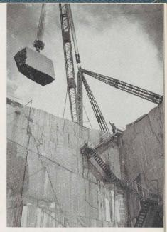
A block of granite, shown above, is raised from the quarry to a waiting truck for movement to the Cold Spring Granite Company, St. Cloud, Minn., to be finished into sections and hauled to Chicago by a GN railway flatbed car, shown below.
