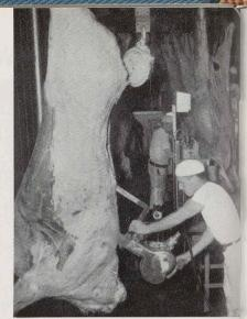
Air-driven knives and saws are used extensively in the new packing plant.
