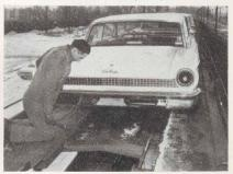
Tie-down chains firmly secure the autos to the rack flooring.
