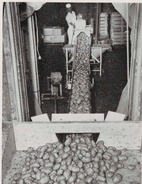
A wheel-mounted motor with universal jointed shaft at side of the warehouse conveyor illustrates power driving car chain conveyors. For unloading, opposite end of car motor is rolled to opposite side of warehouse conveyor and drive is reversed.
