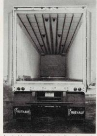
An inside view of the trailer shows the six finger neoprene nylon air ducts on the inside roof assuring good air distribution throughout the cars.
