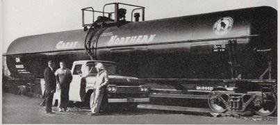
A load of 23,000 gallons of cresylic acid from North West Petrochemical of Anacortes, Wash., is shown shortly before shipment to the Celanese Chemical Corporation in Gallipolis Ferry, W. Va. The car is one of 50 delivered to the GN in 1962. It is approximately 59 feet long, 10½ feet wide and 15 feet high and features a 6-inch gravity discharge outlet. The equipment has heater coils and 100-ton capacity trucks.
