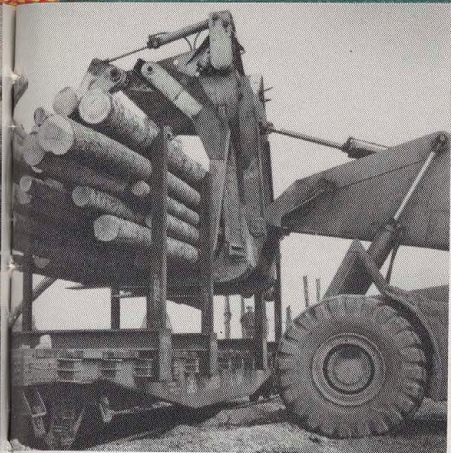
A fork-lift operator easily lowers a load of logs onto one of Great Northern's new logging cars, shown left, above. Bunks on the floor of the car facilitate loading and unloading. A typical loaded car is shown at right with steel posts and pockets securely holding logs.
