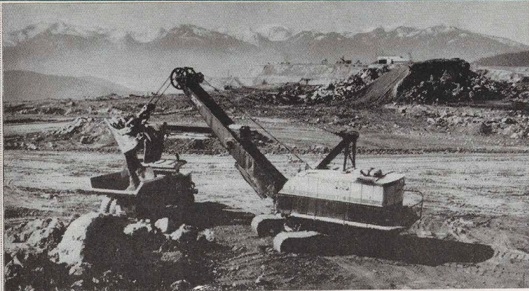
Huge power shovel employed in loading trucks with ore. Snow-capped mountains in the background.
