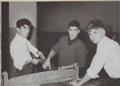
A shearer is utilized to cut metal to workable lengths and widths.
