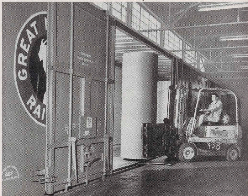
One of Great Northern's new 60-foot long, 90-ton capacity boxcars, equipped with cushion underframes, is being loaded with paper from the St. Regis Paper Company, Tacoma, Wash., for shipment to Los Angeles. The car contained 121 rolls of paper with a weight of 135,538 pounds. The railway has 50 cars of this type.
