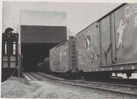
Great Northern boxcars move off land-based tracks, onto ramp tracks and into the hold of the ship which can carry 56 cars.
