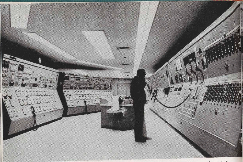
Practically all operations of the concentrator are controlled from this central control room—a complex, electronic nerve center. A television receiver depicts ore in the stockpile.
