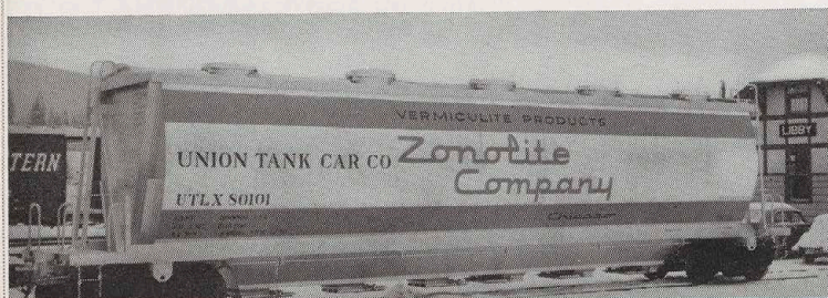
A Union Tank Car Co. aluminum-covered hopper car, shown at Libby, is typical of the type used to haul vermiculite.
