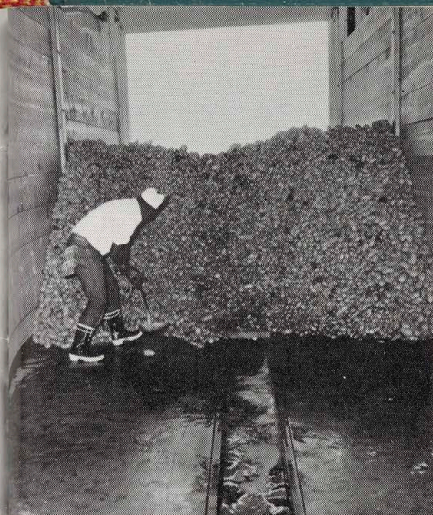
From one of four in-plant storage bays, potatoes are moved via flume into the dehydrating production line.
