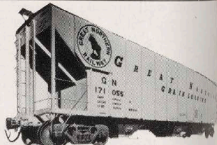
GN "high cube" covered hopper cars haul almost double the grain tonnage of a conventional 40-foot boxcar.
