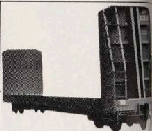
GN bulkhead flats, with tie-down chocks, cushioning devices, ease loading-unloading of packaged lumber and related commodities.
