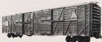
GN 60-foot, "piggy cars"—with upper and lower decks, center gates, shutters and four compartments—haul 250 hogs or 225 sheep.
