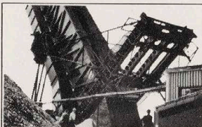
GN end-door gondolas can be upended to dump 90 tons of wood chips in five minutes—and save thousands of man-hours per car, per year.
