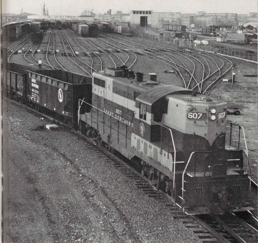
Locomotive pulls cars up the hump from receiving track. Cars will be pushed back over the hump and roll to proper classification track.
