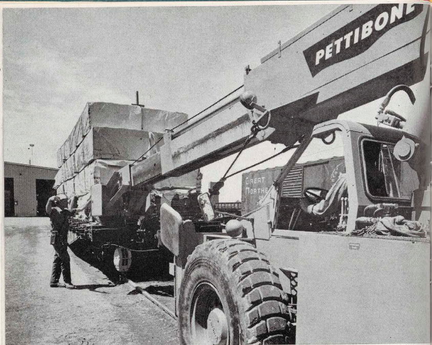
In the event a load requires shifting, the boom is extended and the pusher plate adjusts the load. Ability of the mover to operate from any side of the load reduces adjustment time.
