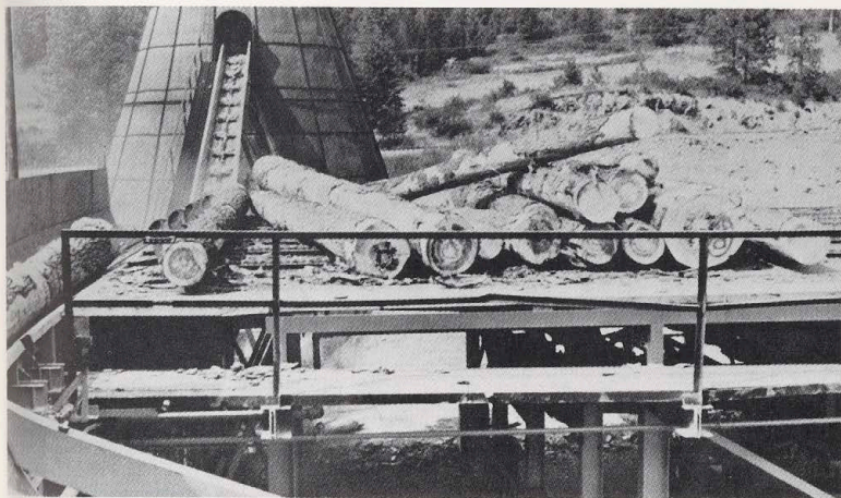
Note low quality of hemlock logs which are only suitable for chipping purposes. Logs pass additional sorting facilities before being committed to the chipper.
