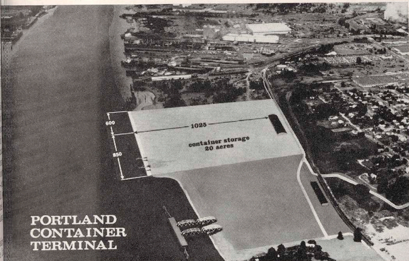
Portland Container Terminal, under construction, will include a 35-acre automobile receiving terminal with floating dock (foreground).
