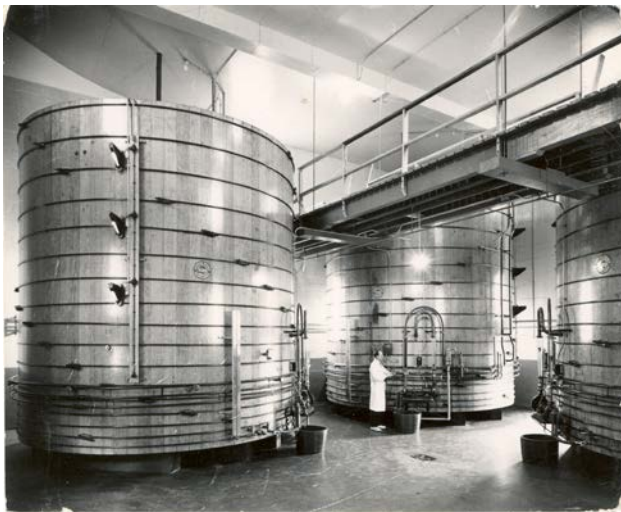
These generators were eventually moved to Chaska in 1991 and later joined by two even more state-of-the-art "acetators", using high powered oxygenators in small fiberglass tanks that could triple the efficiency of these generators.
