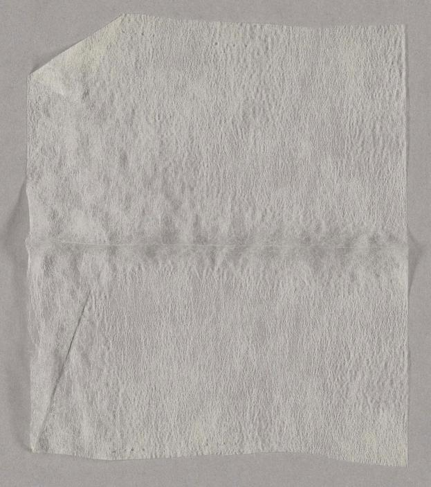
27678 77679. 11/25/44 Lens Tissue for lens cleaning jumposes a combination of carded trasme with absorbent punched trasme with absorbent meneral of carded tirene 2. I'mil toilet tisme 2,5 mil down a hot flate at heaten 380° F. good bond obtained at place where solvent & heat were in right legace, allowed improved. Some increase in lint seems to have been occasioned. Sample #77678 is attacked. If possible a less linty absorbent tissue will be obtained for use. 4.2, midl 11/25/44
