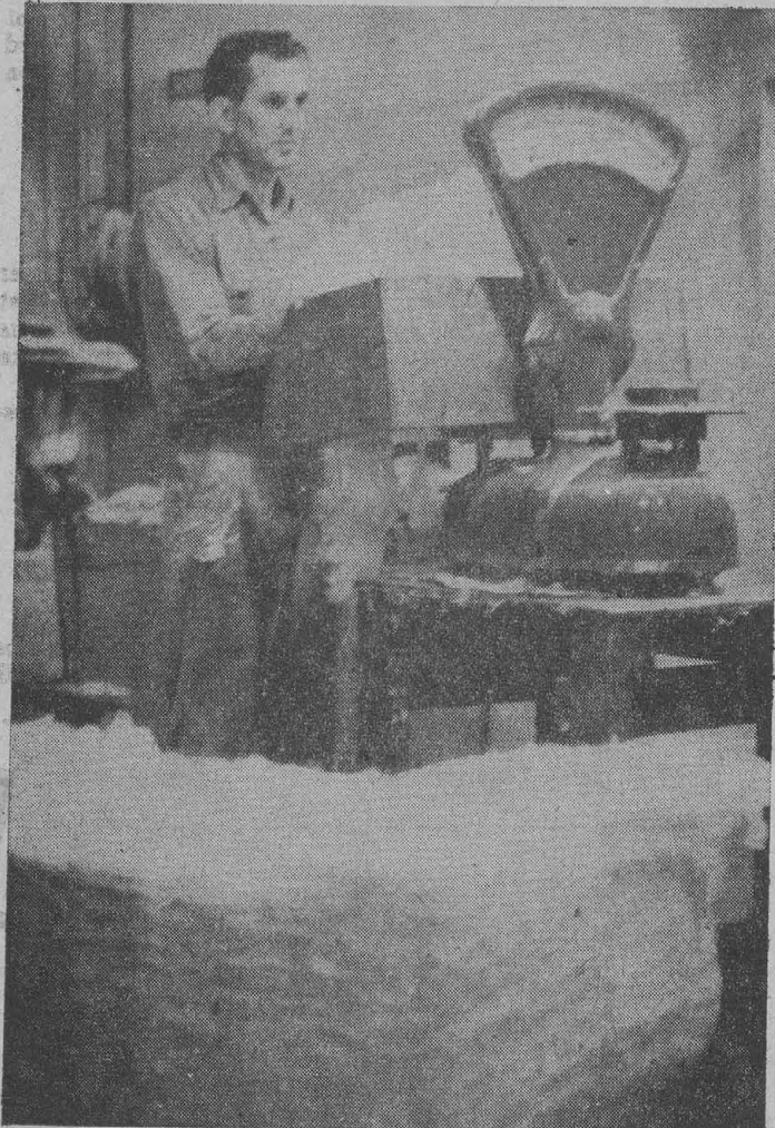
WEIGHING IN RAW MATERIALS — Richard Dyslin weighs acetate and viscous fiber, the cellulose materials used for manufacture of the rolls of ribbon. The material, which comes in big cartons, is purchased by the plant. In turn, the raw material is fed into the garnett machine, a common fixture in the textile industry which transforms the raw material into a web.
