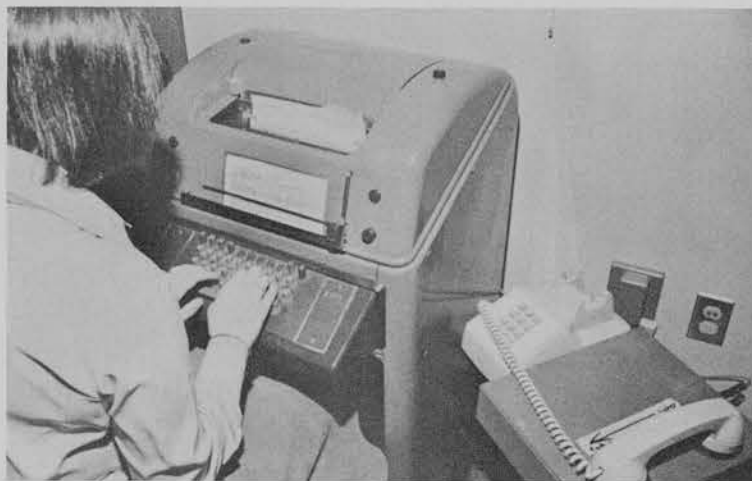
The teletypewriter permits typewriter-telephone hook-ups, allowing typewritten messages to be transferred via the telephone line. Messages are received in typewritten form on either end of the line.
