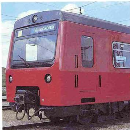
Trains for local traffic around Copenhagen, Denmark. ASEA has supplied all the electric equipment including chopper control.
