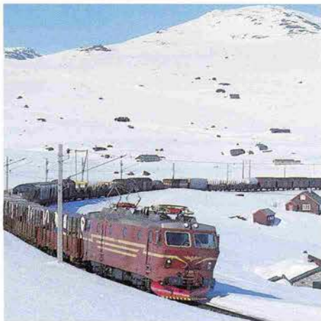
Locomotive EI 16. With its 4400 kW and thyristor control equipment, it is probably one of the world's most effective 4-axle locomotives.
