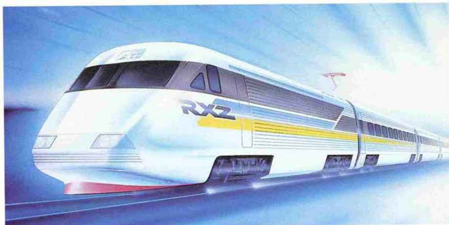
Proposed high-speed train for the Swedish railway main lines. Controlled tilting of the cars allows the train to run through the curves at higher speed whilst maintaining full comfort for the passengers.
