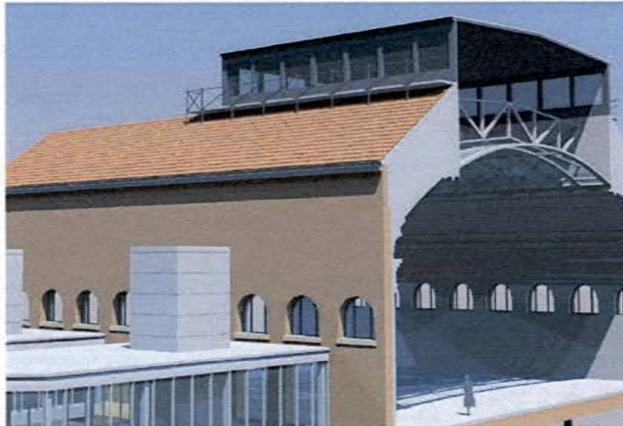
WAITING ROOM ROOF WITH CLAY TILES
