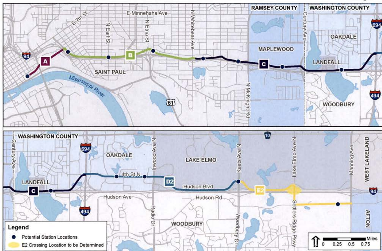
Figure 1 shows the recommended alignment for the Locally Preferred Alternative in the in the Gateway Corridor. The recommended mode is dedicated bus rapid transit.
