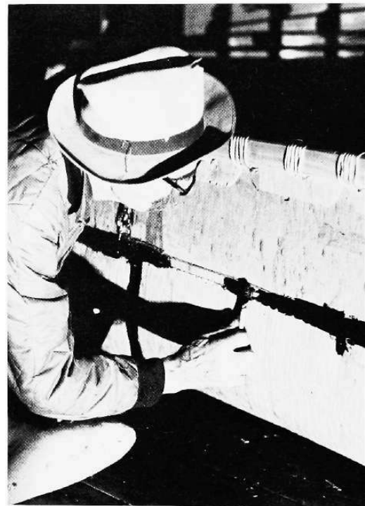
MORE RIBS are pounded into place.
