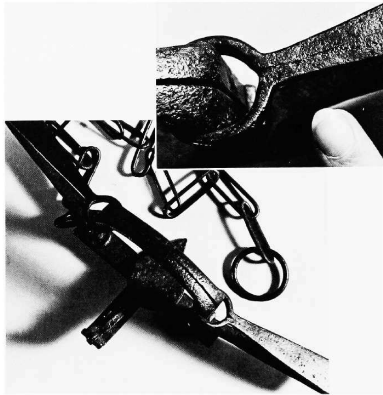
AN EARLY NEWHOUSE trap, which probably dates back to the 1840s, is remarkably similar in design to modern traps. Note the hand-forged details on the jaw and spring in the inset photograph.
