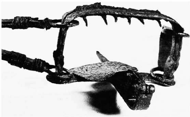
SEVERAL TEETH, fastened with leather or a similar material, were added to this beaver trap so that it could be used to catch otters.
