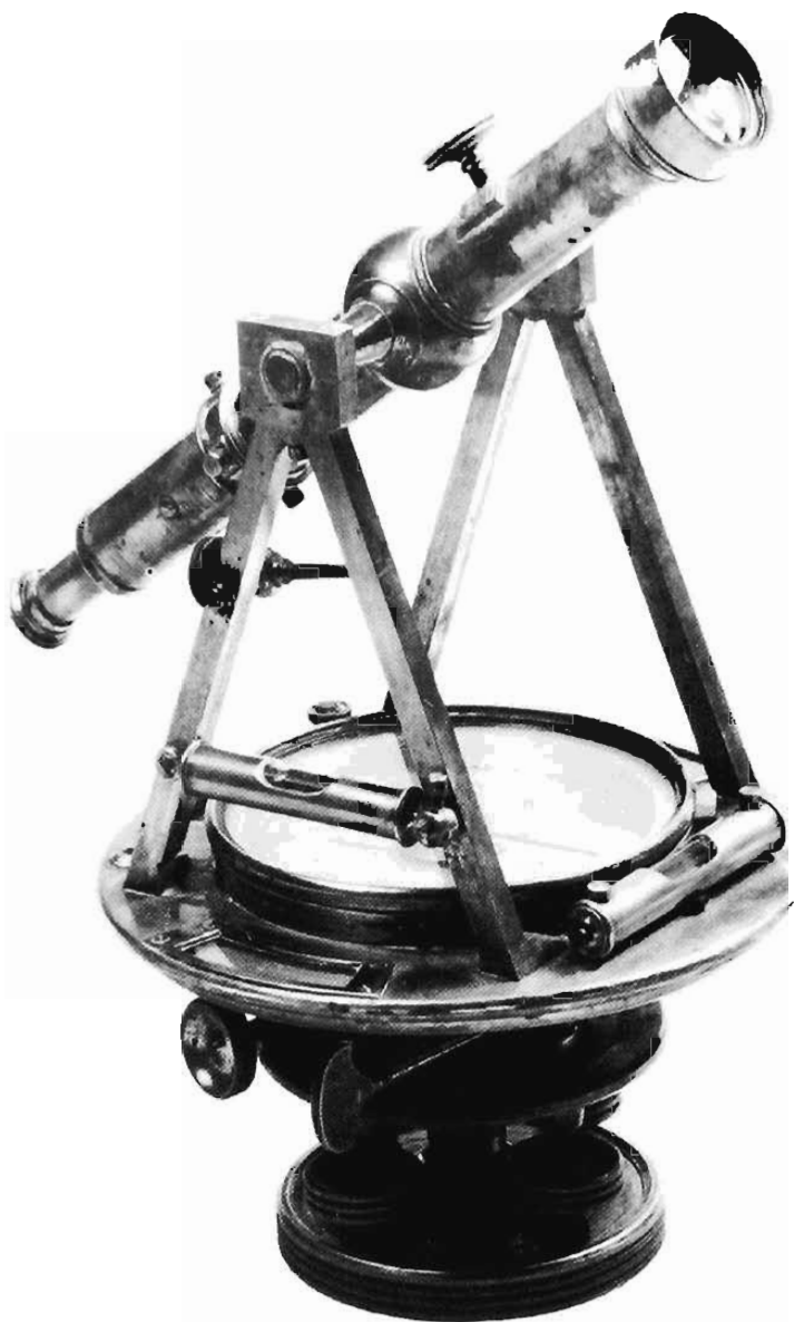
Portable surveyor's transit, used from 1853 to 1900 in Stearns County
