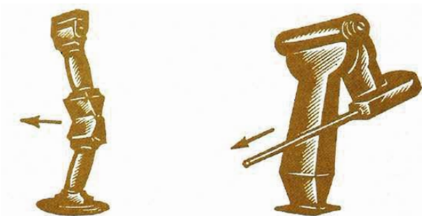
Equal-length levers, characteristic of the Smith press knee-joint (left), and the improved "figure 4" design of the Washington
