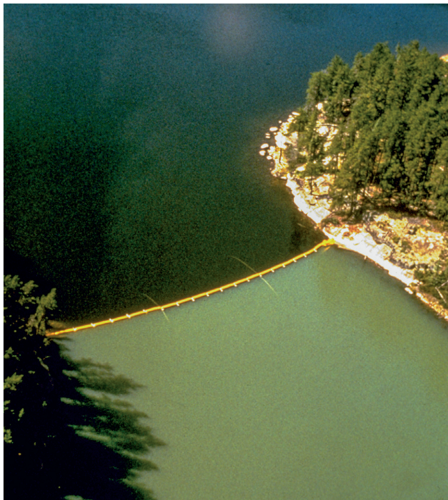
A plastic curtain was placed across a narrows in Lake 226 in the Experimental Lakes Area, and phosphorus (then commonly used in detergents) was added to one side of the lake. The algal bloom that developed on the phosphorus side (bottom of photo) provided dramatic evidence of the effects of pollutants on our lakes and waterways.
