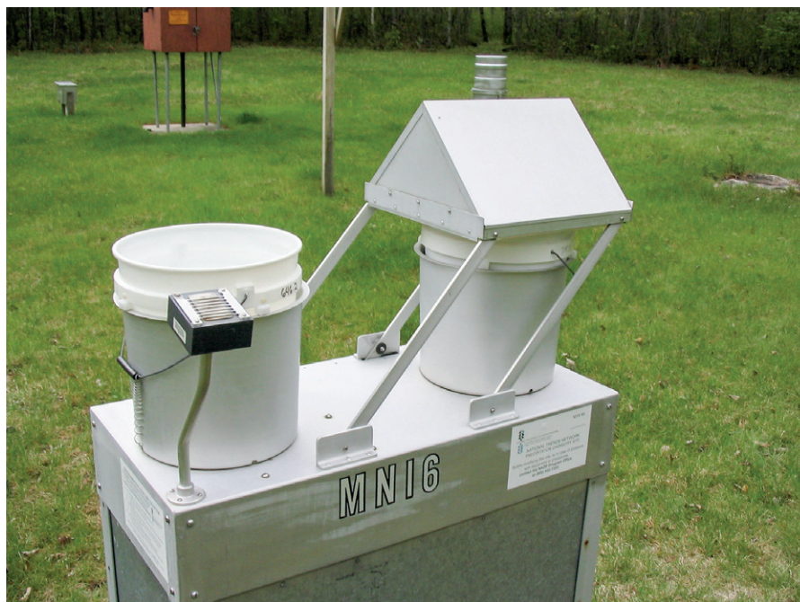
This two-bucket type of rain sampler began to be used widely in Minnesota and around the country in the 1970s. The precipitation detector on the front triggers the cover to move across to the second bucket, allowing precipitation to be collected in the bucket on the right.
