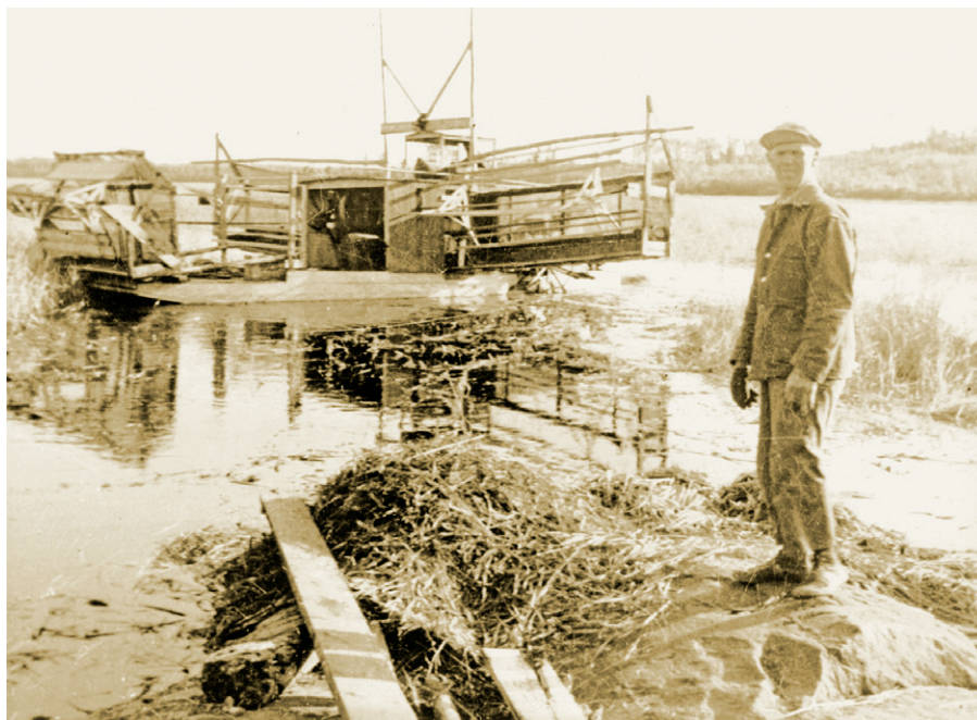
A paddle wheel harvester that could pick a bag of wild rice per minute, circa 1930
